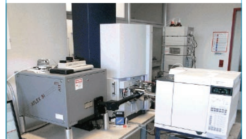
APLI source coupled to a microTOF II™ (Courtesy of Bruker Daltonics™)
